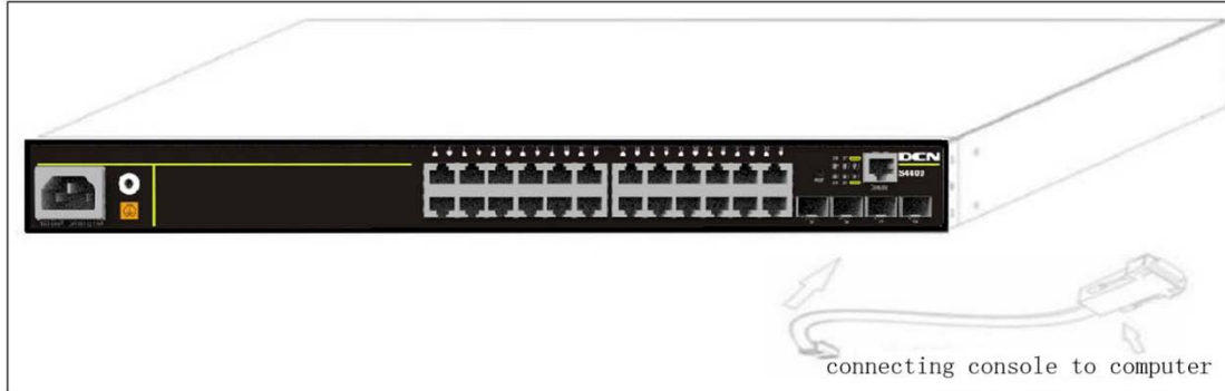
Fig 2-3 Connecting Console to switch
