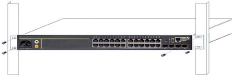
Fig 2-2 Fasten the Switch to the Rack
